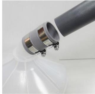
3. Use a slotted screwdriver to tighten on two hose clamps.
